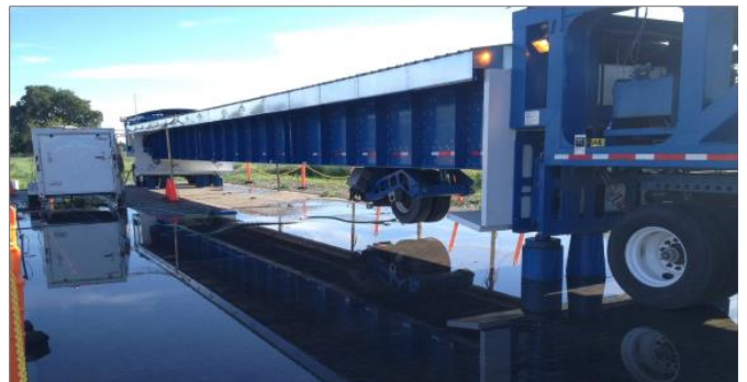
Permeable pavement testing equipment
