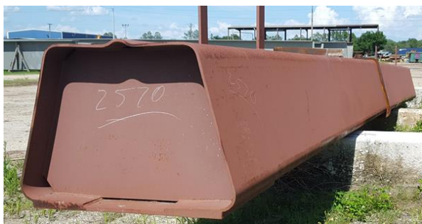
SPGS test specimen prior to deck prefabrication
