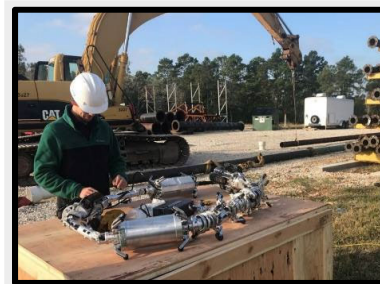
In-Line Inspection Technology for Small Diameter Pipelines (Courtesy of Quest Integrated, LLC)
