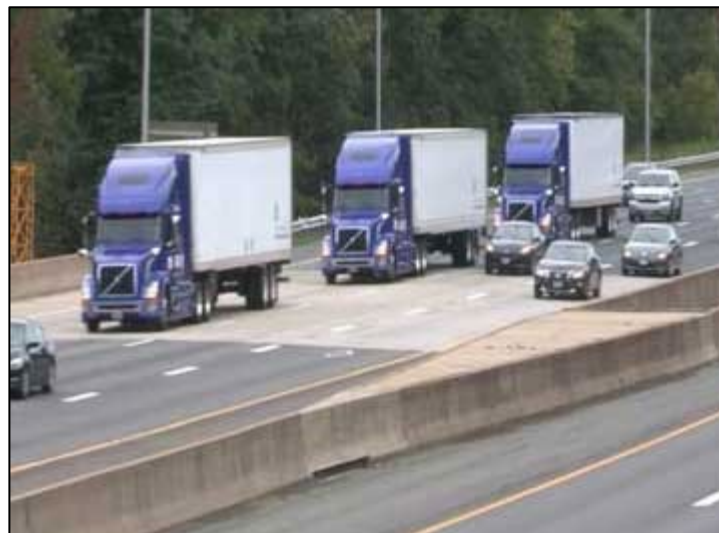
Figure 11. Demonstration of three-truck platoon on I-66 in northern Virginia.
