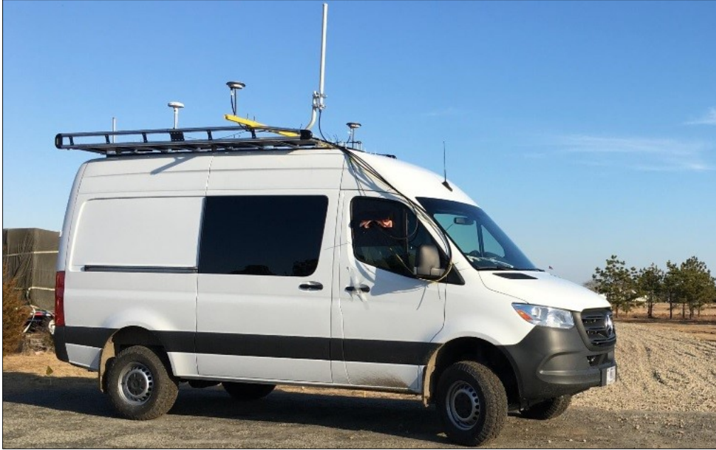
Figure 21. Rover Subsystem with Antennas as Installed in Sprinter Van at JBCC
