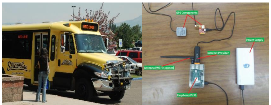
Streamline bus containing Smart Station device (left) and components of the Smart Station data collection system (right)
