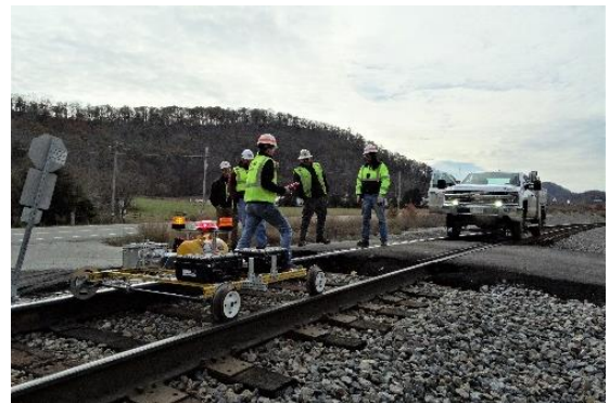
Prototype Rail Lubricity Instrument during a field test on revenue service track
