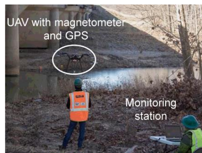
Magnetic measurement with a UAV-based sensor
