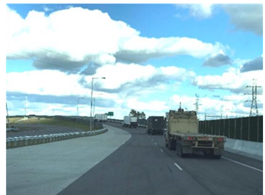
Platoon of 4 semi-trucks: lead truck is manually driven, the rest are CAVs
