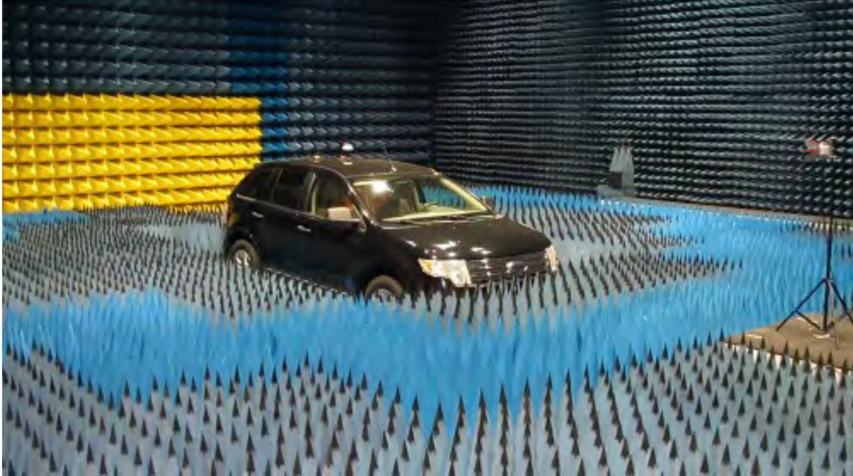
**Figure 6-8: Antenna pattern measurement on test vehicle in a CERDEC anechoic chamber**
