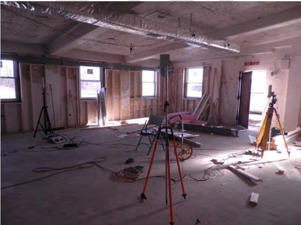
Figure 10-22. Brick building with the surrogate UNII-4 interferer set up inside
