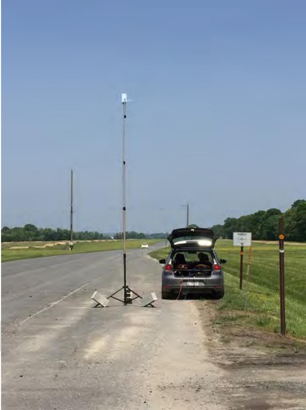
**Figure 7-4. UNII baselining – client on 18’ tripod, access point in white vehicle at Perryman test track**
