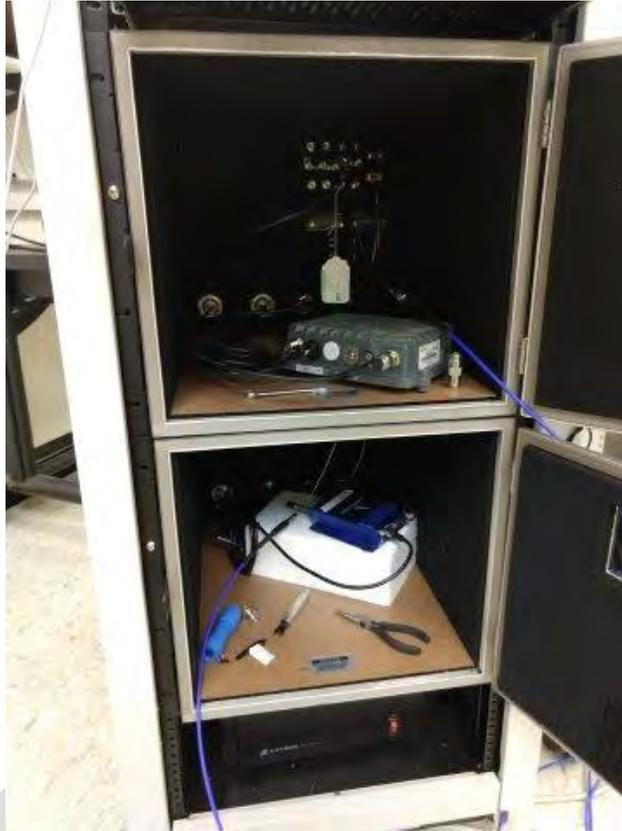
Figure 6-2. RF Enclosures for calibration at ITS Boulder
