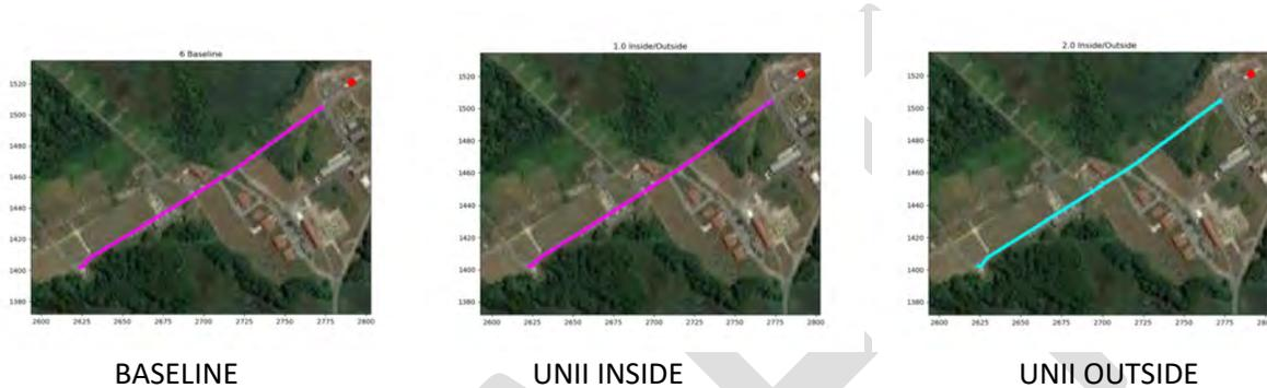
**Figure 10-40. Geographical distribution of PER, I2V, UNII EIRP=35 dBm, 70% load, departing Brick building**
