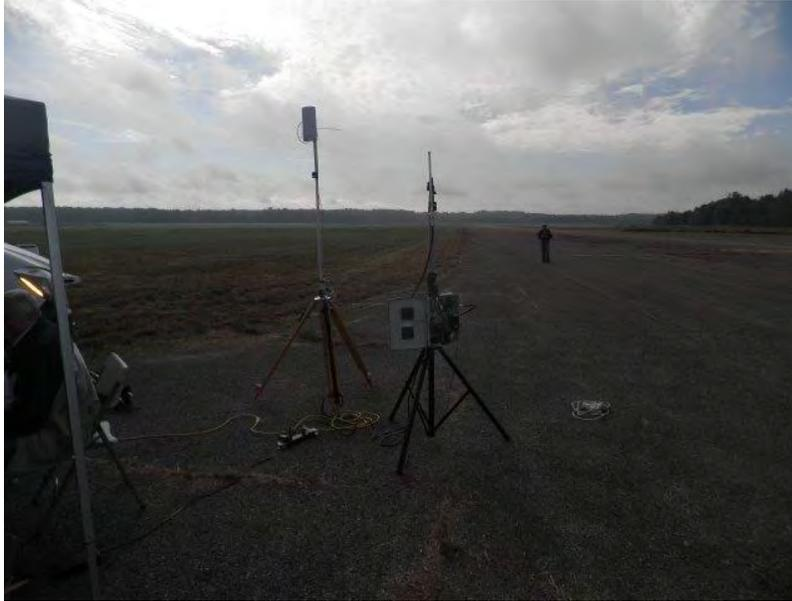
**Figure 7-13. Interferer set up as outdoor access point and client at Zone 1**
